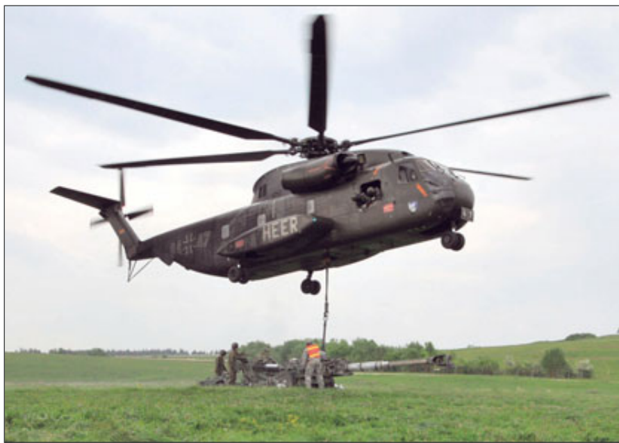
Bulldog Battery, Fires Squadron, 2nd Cavalry Regiment Soldiers hook two M777A2 howitzers to a German CH-53 Stallion helicopter during an artillery raid operation in the Grafenwoehr Training Area.
